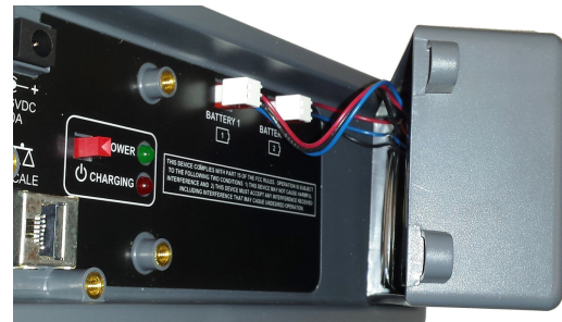
Battery pack connections
