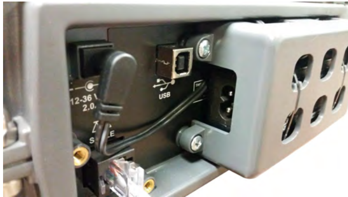
Figure 2.6 AC power block
