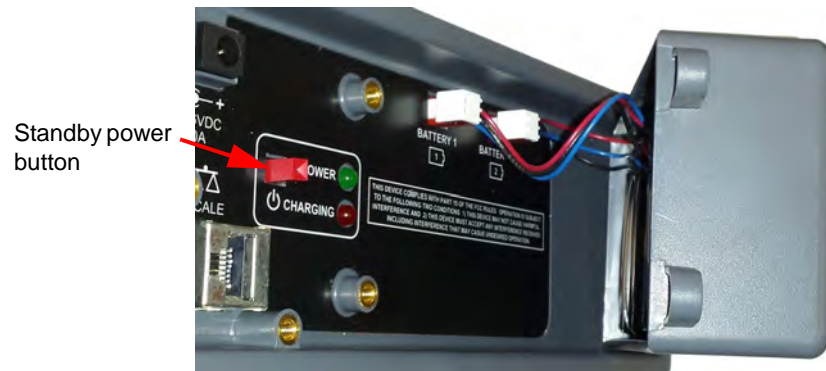
Figure 2.8 Battery pack connections
