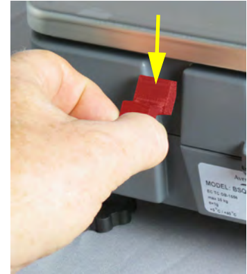
Slide the stop down and remove it from the slot. Keep for future shipping.
