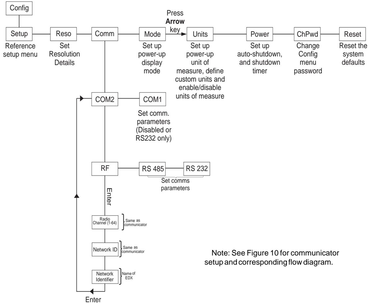
Note: See Figure 10 for communicator setup and corresponding flow diagram.
