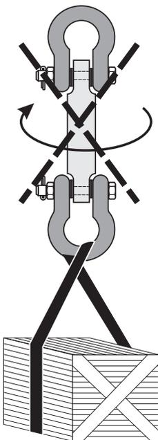
Do not torque, bend or side load.
