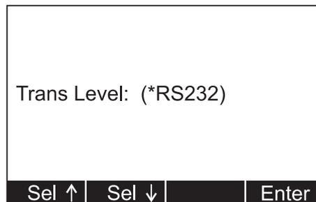
3. Select a transmission level using the **Sel** keys to scroll through the four choices; Disabled (default), RS232, RS485, and RF. RF stands for Radio Frequency and means transmission would be by radio (requires optional radio board). Press **Enter** to accept the setting. See note at left.
