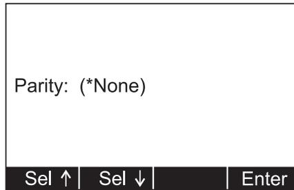
5. Select a parity value using the **Sel** keys to scroll through your choices. Choices are none (default), odd and even. Press **Enter** to accept the setting.
