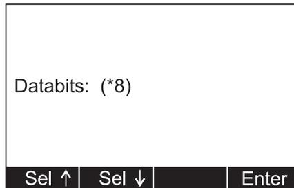
6. Select a databit value using the **Sel** keys to toggle between the two choices; 7 or 8 (default). Press **Enter** to accept the setting.
