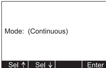
7. Select a mode of communication you want using the **Sel** keys to scroll through these choices; Continuous, Poll, Remote and Print Key Only. Press **Enter** to accept the setting.
